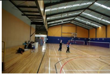
Circulation between edge of court to plat seating appears sufficient (max. of 2.0m)
