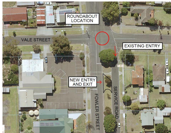
Figure 1 – Existing and Proposed Service Road Entrances
