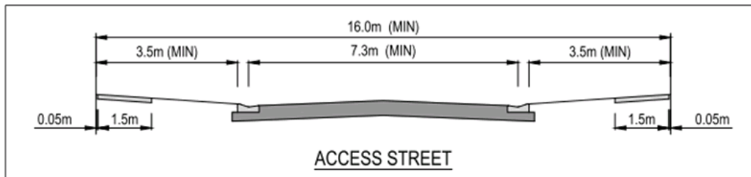
Figure 5 Cross Section – Access Street
