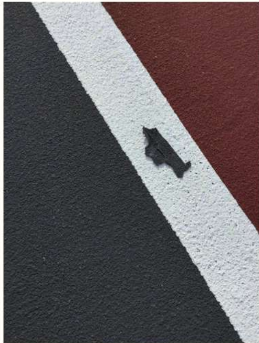
Piece of delaminated acrylic sitting on the court surface. The sample confirms that the delamination has not affected the Qualipur.
