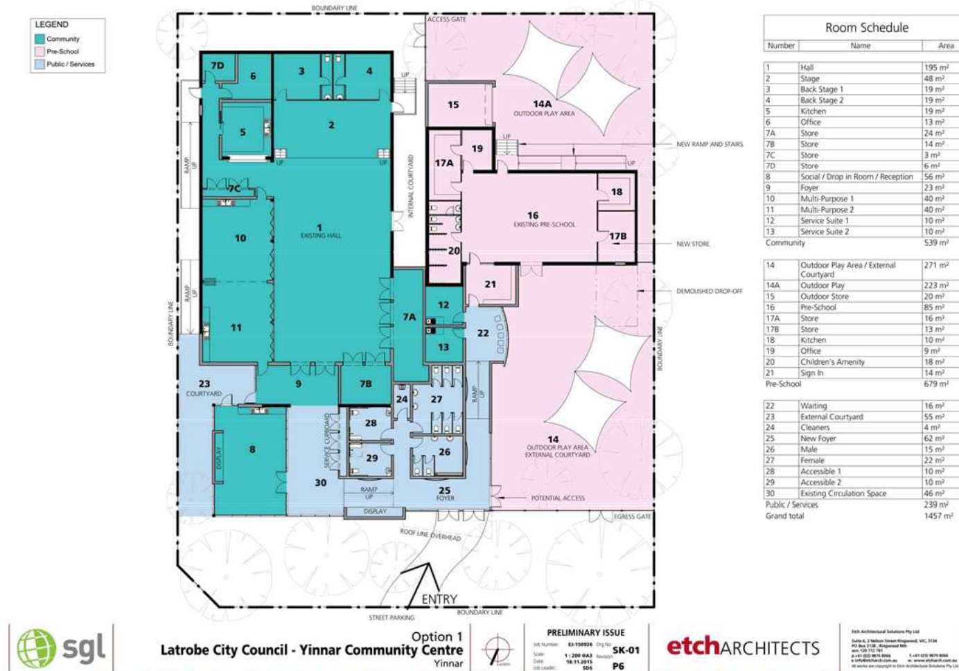
Figure 3.1 Option One: Redevelopment of Yinnar & District Memorial Hall and Pre-school into the Yinnar Community Centre
