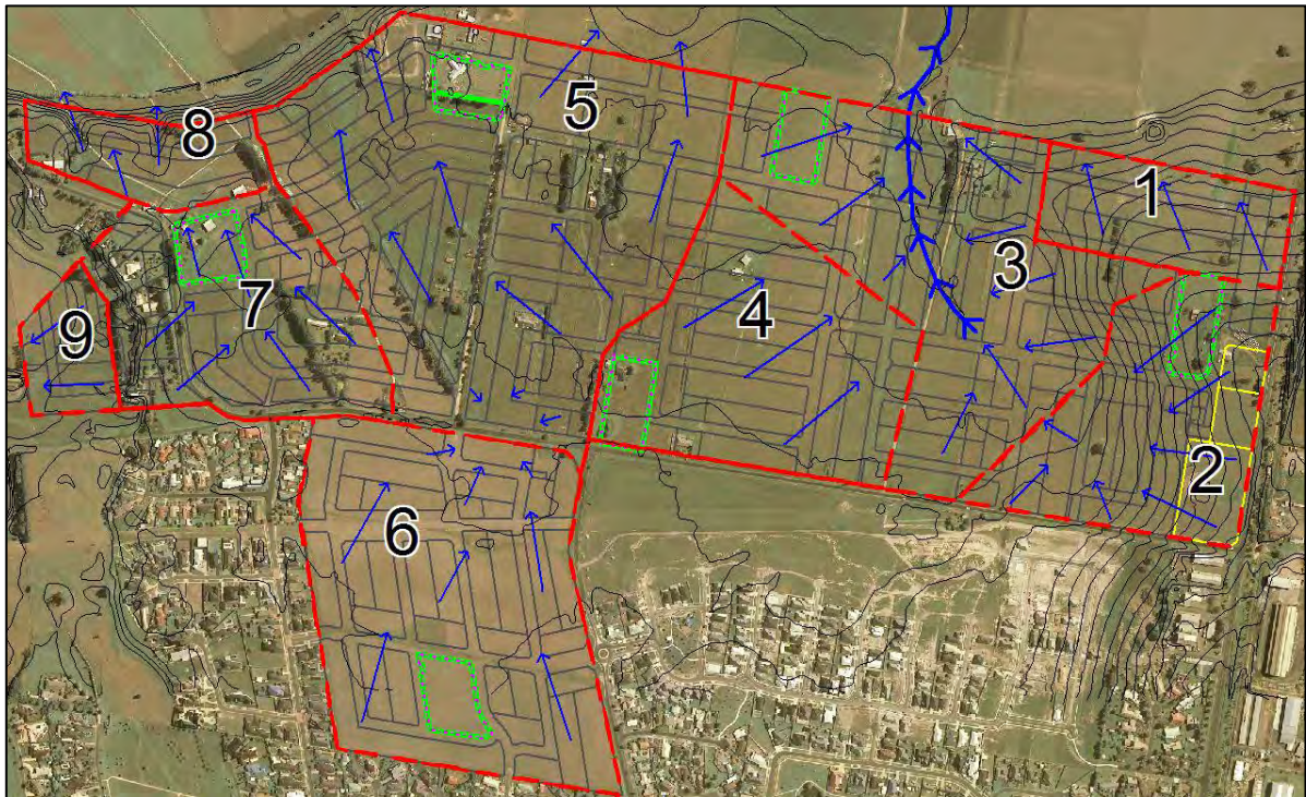
Figure 3-1 Existing (undeveloped) drainage characteristics
