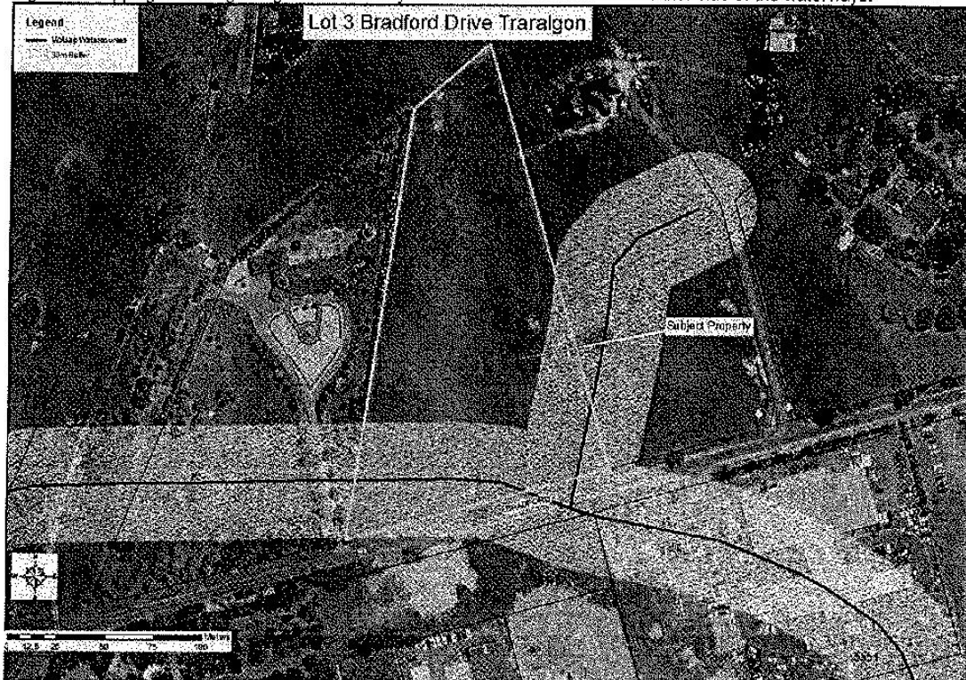
Figure 1: Mapping indicating designated waterways and 30 metre buffer zone on either side of the waterways.
