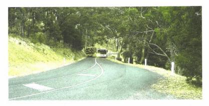
The log truck had to put its wheels in the unsealed gutter to squeeze past the school bus. A rear wheel of the bus is on the narrow, unstable verge beside a drop-off.
