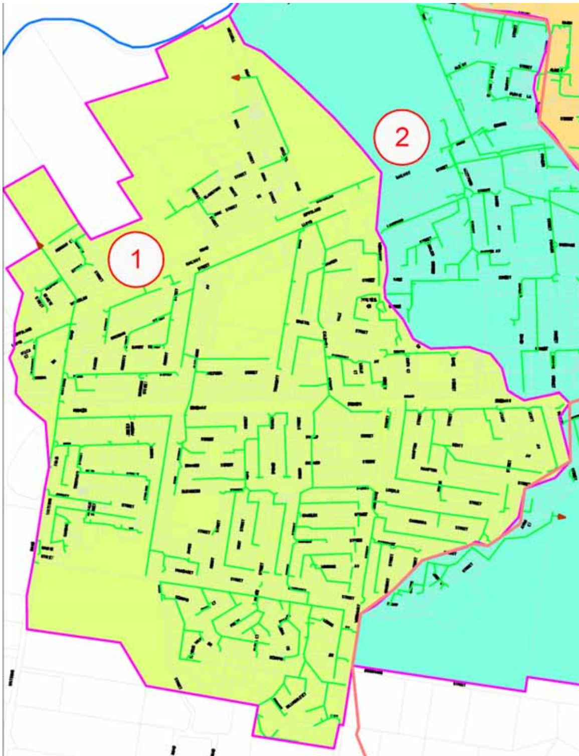
Figure 3 Extract from LCC SWMP (Fisher Stewart 2001) showing pipeline layouts in the Moe Contour Drain (west) catchment.
