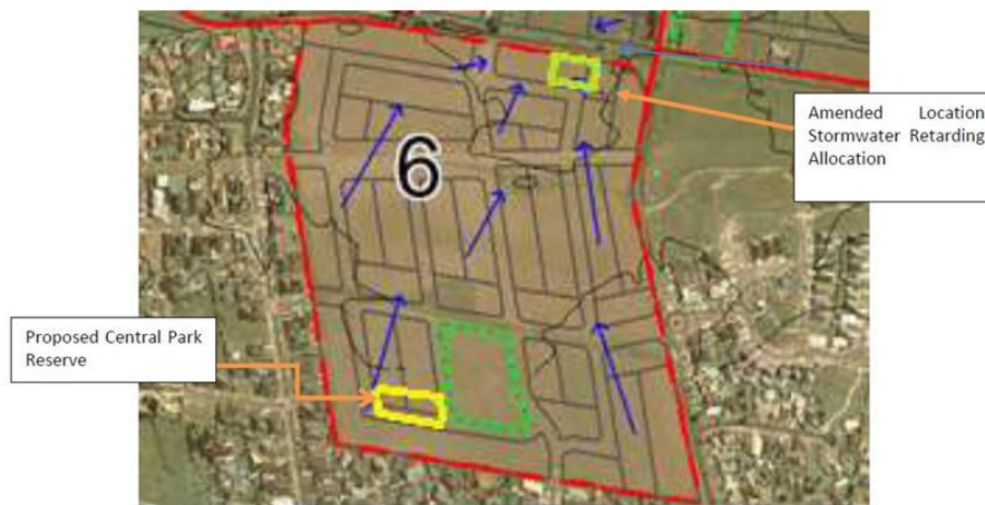
Figure 6 - Existing undeveloped drainage characteristics
