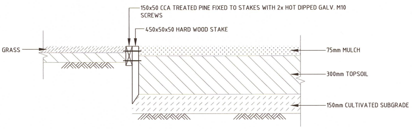
TIMBER EDGING DETAIL NOT TO SCALE
