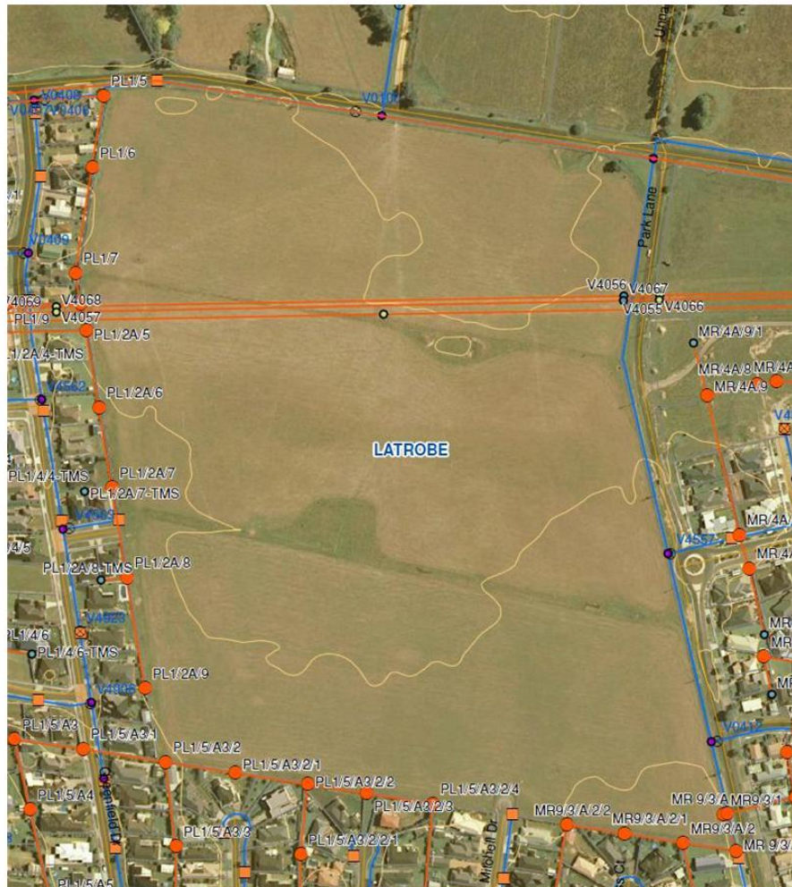
Figure 4 - Sewer Asset Plan
