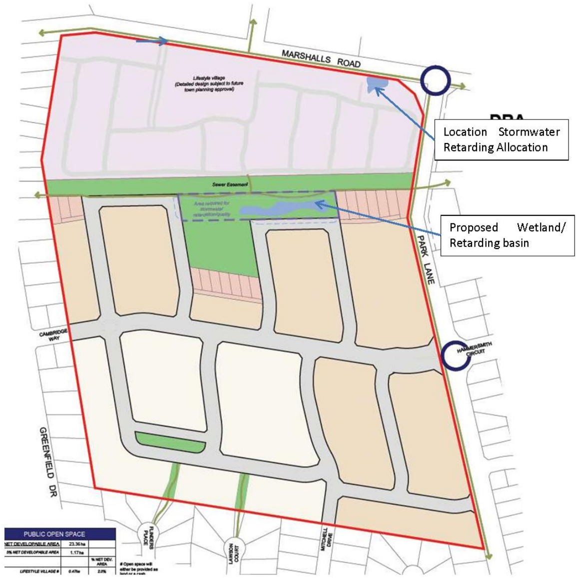
Figure 3-3 Revised - Likely developed conditions drainage characteristics and proposed features
