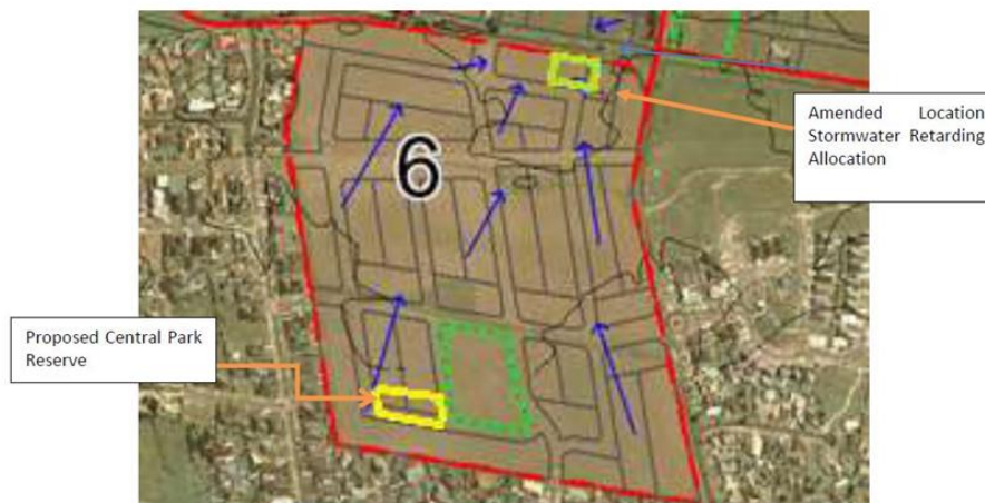
Figure 6 - Existing undeveloped drainage characteristics
