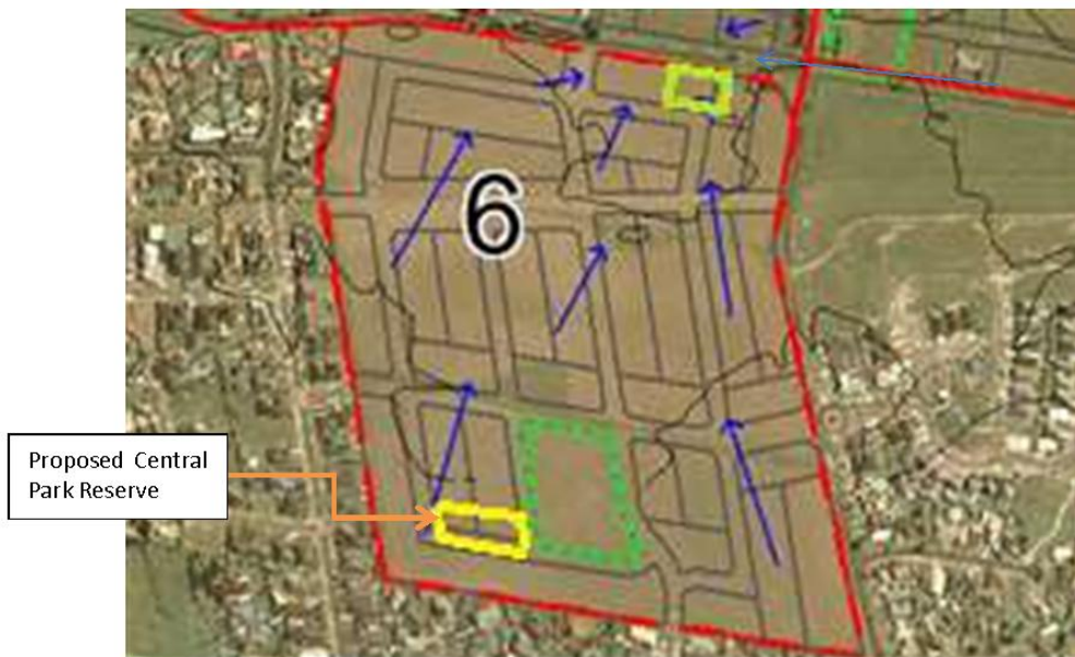
Figure 3-2 Existing (undeveloped) drainage characteristics Catchment 6.
