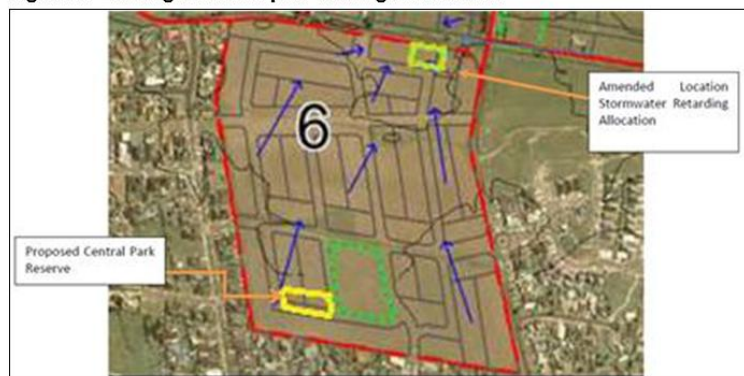
Figure 4: Existing undeveloped drainage conditions
