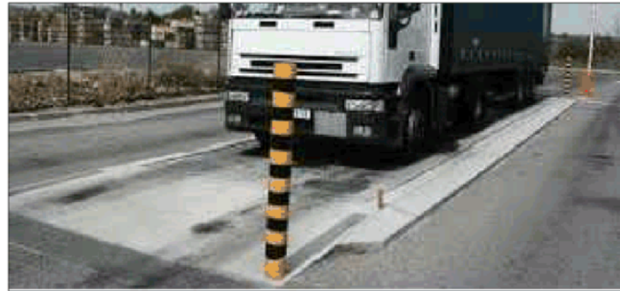
TYPICAL WEIGH BRIDGE 100 TONNE CAPACITY
