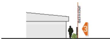
Section illustrating side setback comprising path and landscape belt
