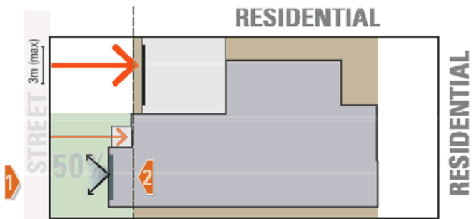
Example of site planning and front setback arrangement in a limited or minimal change area
