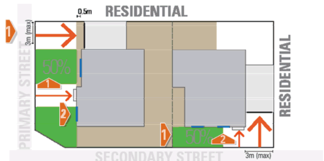
Example of site planning and front setback arrangement in a limited or minimal change area
