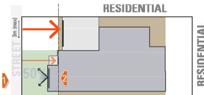
Example of site planning and front setback arrangement in a limited or minimal change area
