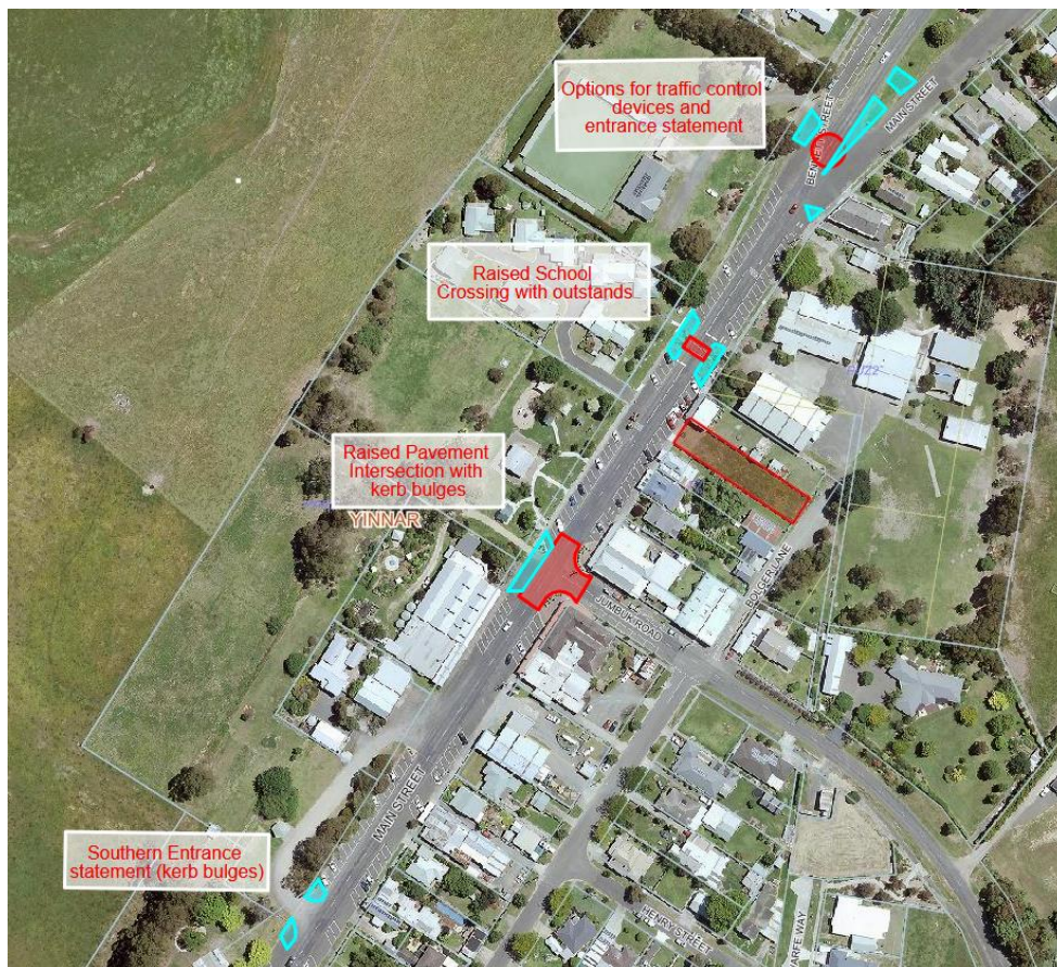
Figure 2 – Main Street potential physical traffic calming measures
