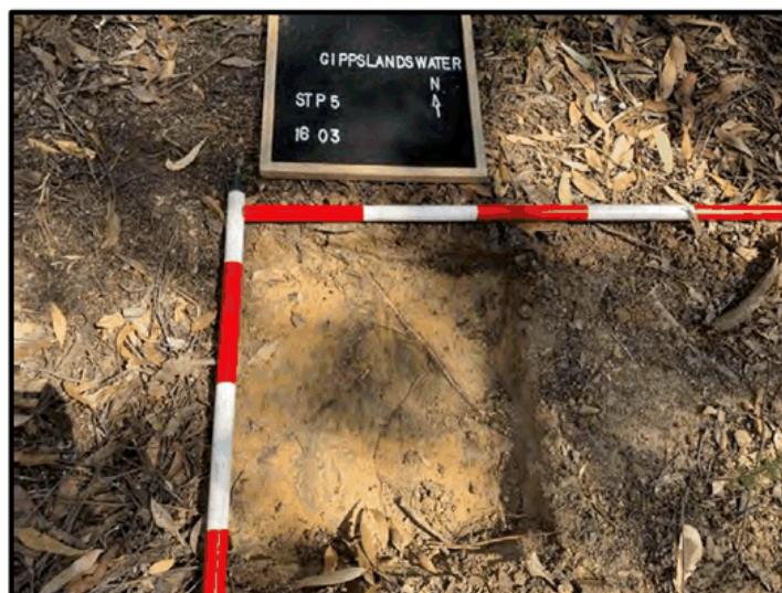
Plate 18: Photo by M. Barker (16/3/20) showing an example of soil profile in Shovel Test Pit 5 with clay on the surface and no silt layer
