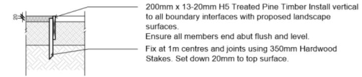
1 Timber Edge Typical Edging Detail 1:20 @ A1
