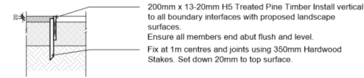
1 Timber Edge Typical Edging Detail 1:20 @ A1
