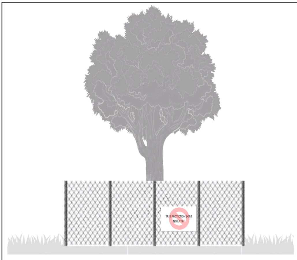
Figure B.B Tree Protection Zone
