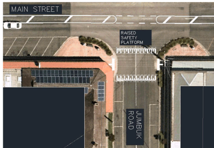
Figure 7 – Jumbuck Rd and Main St raised safety platform
