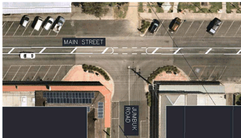
Figure 3 – Painted centre median island
