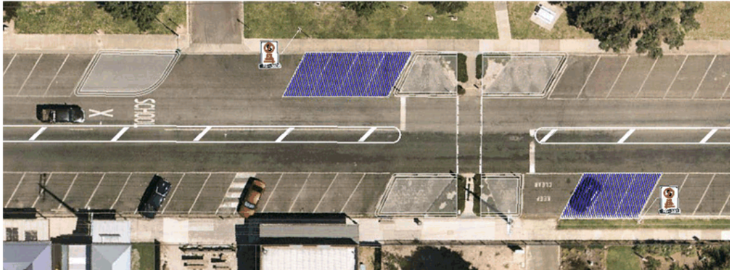
Figure 6 – Main St kerb outstands and school crossing
