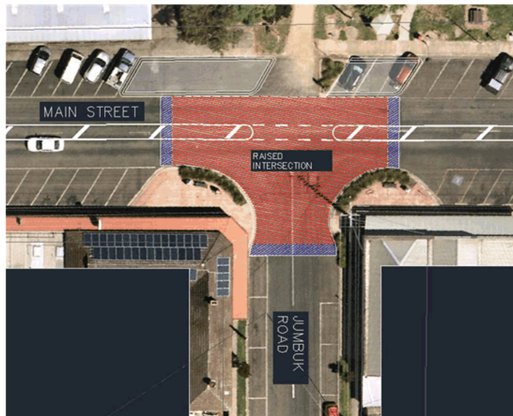
Figure 8 – Raised intersection treatment
