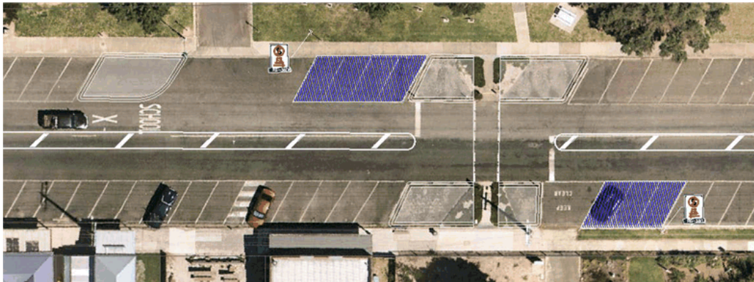
Figure 6 – Main St kerb outstands and school crossing
