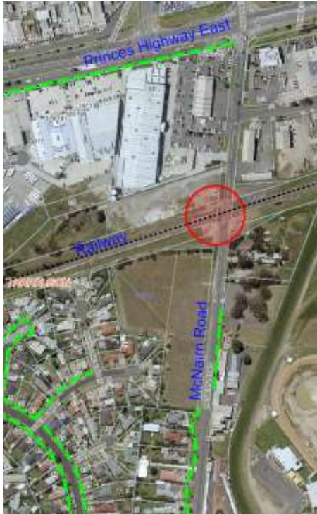
Figure 1 – Location of Proposed At-Grade controlled Railway Pedestrian Crossing. Green dashed lines show existing footpaths
