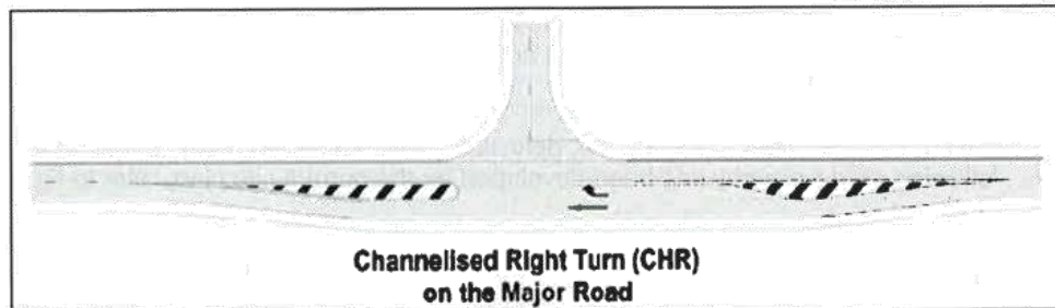
Figure 12 : Rural channelised right turn treatment
