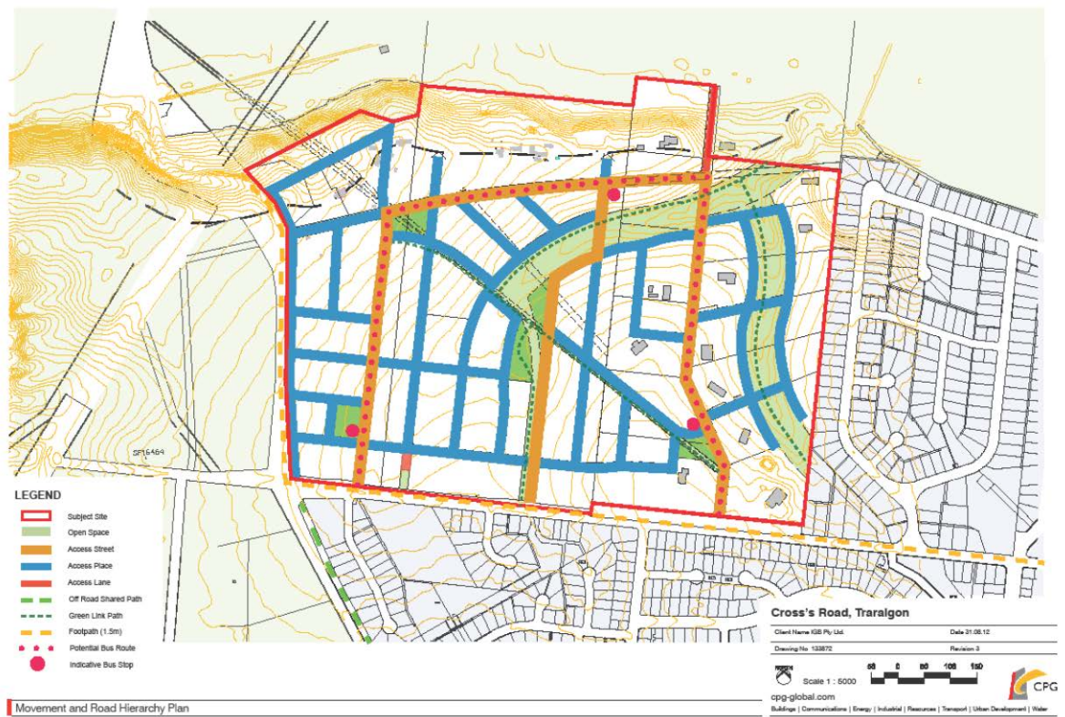
Figure: Extract Figure 9 Street hierarchy and internal and external active path network – Cross's Road Residential Precinct Development Plan
