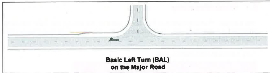
Figure 10: Rural basic left turn treatment
