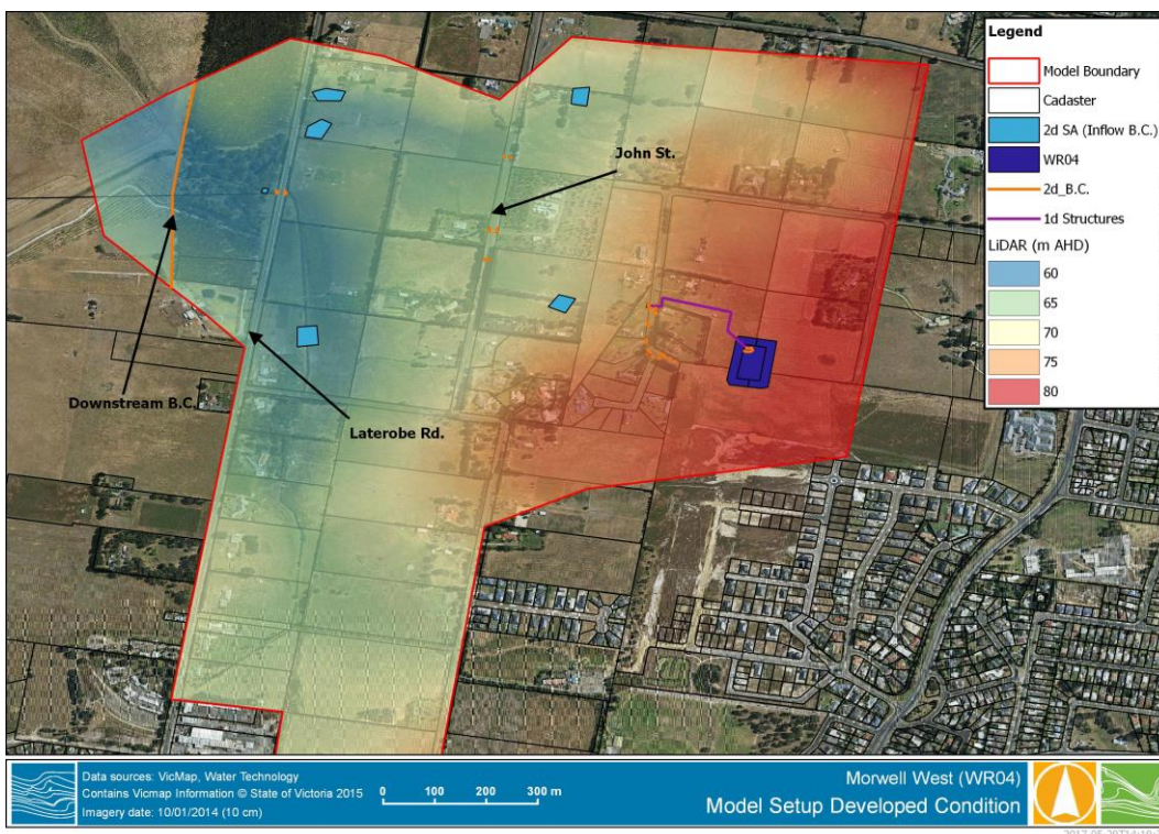
FIGURE A-1 FLOOD MODEL SETUP EXISTING CONDITONS
