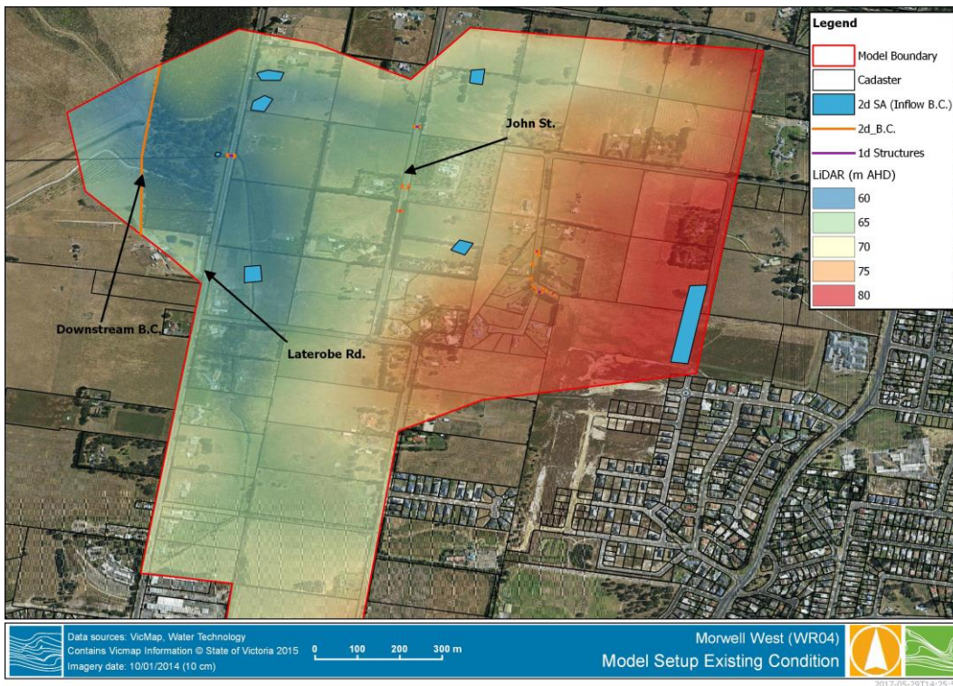
FIGURE A-1 FLOOD MODEL SETUP EXISTING CONDITONS
