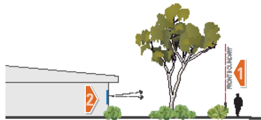
Section illustrating preferred front setback and fence conditions
