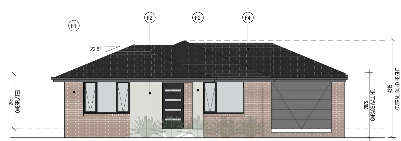
1A LUCAS 12 'ACCESS' FACADE - FRONT ELEVATION 1:100
