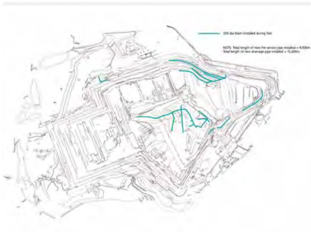
Figure 2.26 Water pipe installed during Hazelwood mine fire 93
