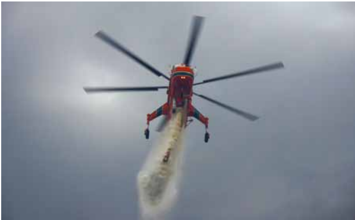
Figure 2.28 Sikorsky helicopters were effective in suppressing fire in steep mine batters
