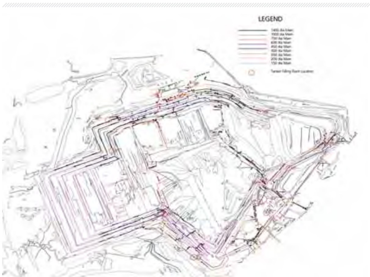
Figure 3.17 Fire service network as at 9 February 2014 154
