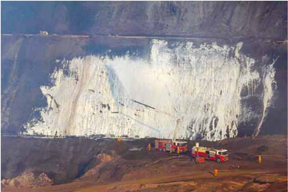
Figure 2.27 The use of compressed air foam to smother batters at Hazelwood mine 111
