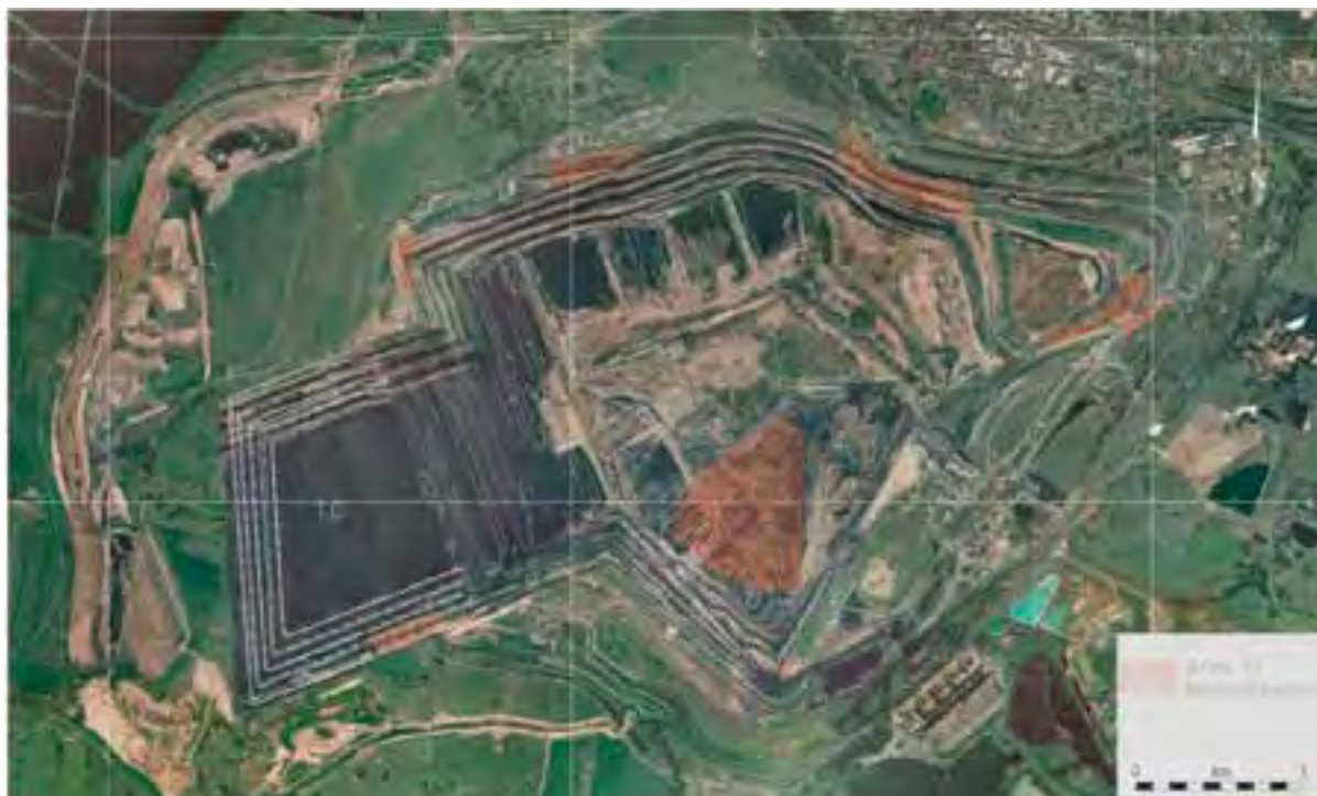
Figure 3.9 Progressive rehabilitation staging/sequencing – rehabilitation at end of block 1C (2019) 43
