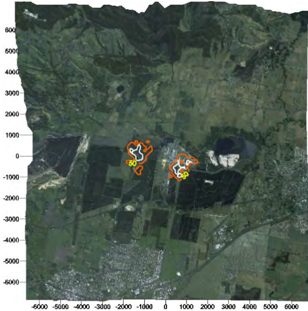
Figure 9 Predicted Return Interval of Exceedence of 5 OU Stack Emissions using AUSPLUME (TRS/odour link of 1.4 ppb = 1 OU).
