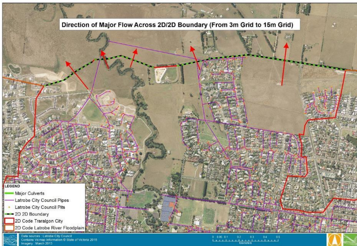
Figure 3-11 Schematisation of the 2D/2D Boundary within TUFLOW
