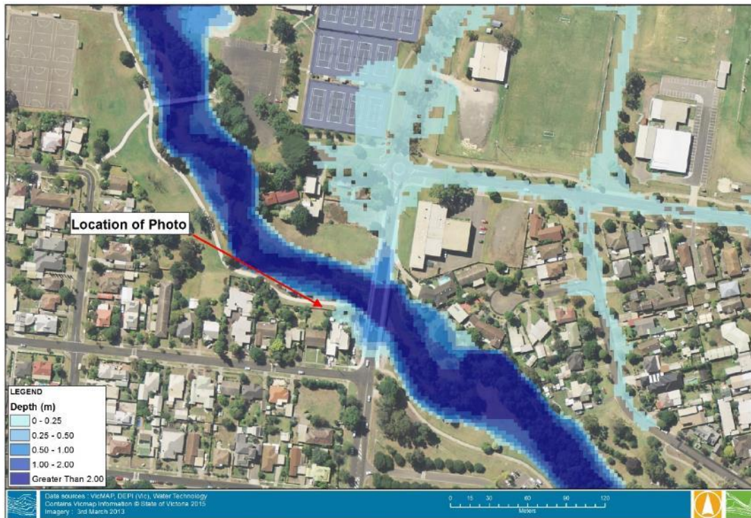
Figure 4-10 June 2013 Flood Depth Plot at Franklin Street
