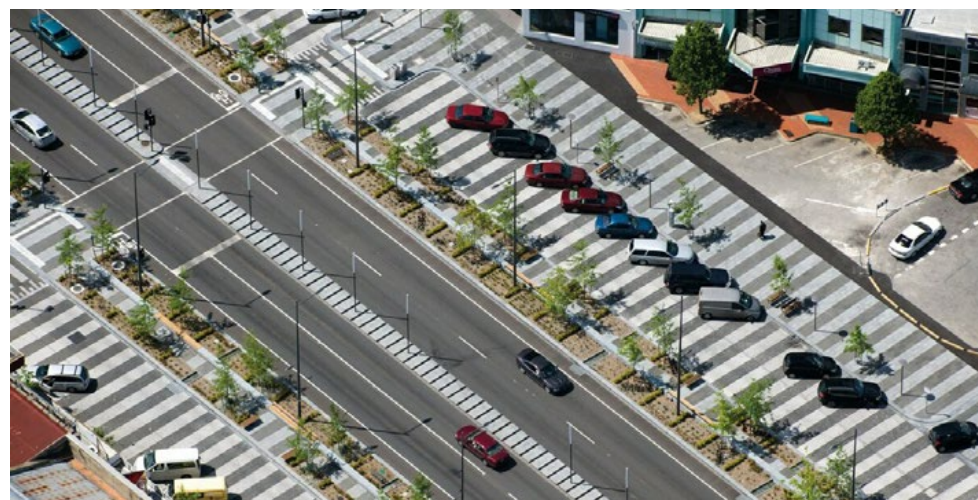
Figure 61: Parking integrated with high quality public realm with pedestrian footpath and crossing priority and spaces for the community to linger at Source: TCL
