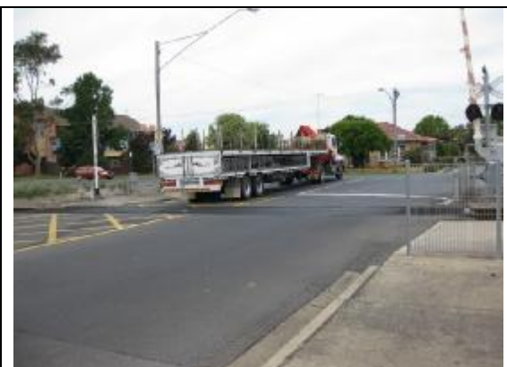
Photograph 6 Semi trailer extending across railway lines when queued at Moe – Glengarry Road intersection.
